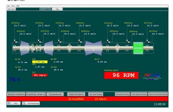
The application has the option of defining several synoptic screens with different images of the monitored process. The buttons at the bottom of the application window allow you to switching between synoptic screens. The current window view can be saved as a graphic file.
